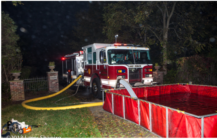
A front mounted suction utilized to draft from a portable pond.
